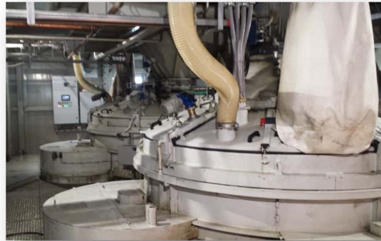
Mixer's platform with 2 countercurrent mixers PGM 2250 / 1500
